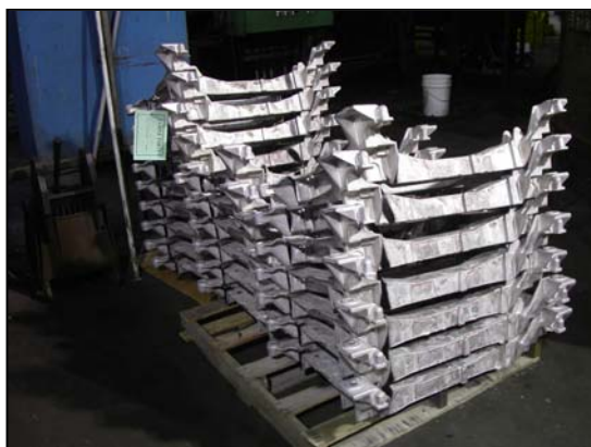
Figure 4. Initial machined HPDC cradle castings
