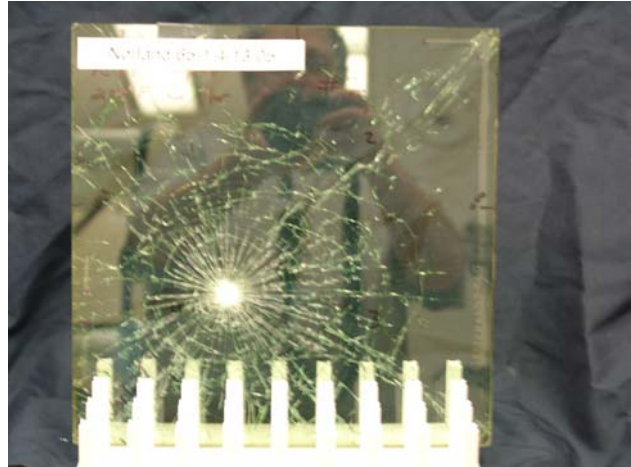
Figure 4. Impact-tested plate with 252 g ball at 9.14 m.
