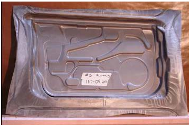
Figure 4. Inner door panel warm formed using refitted steel stamping die.
