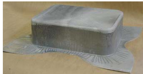
Figure 5. Deep-drawn panels warm formed using a purpose-built warm-forming die.
