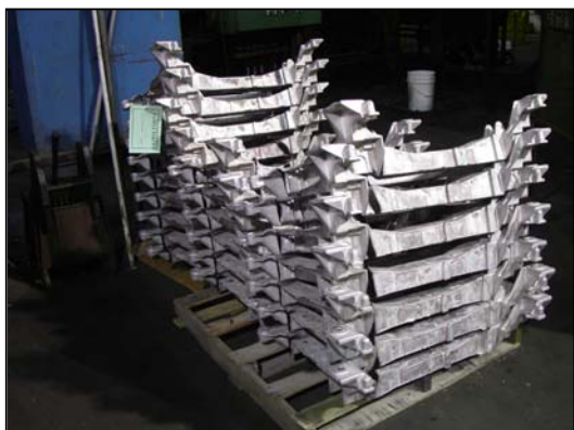
Figure 4. Initial machined HPDC cradle castings.
