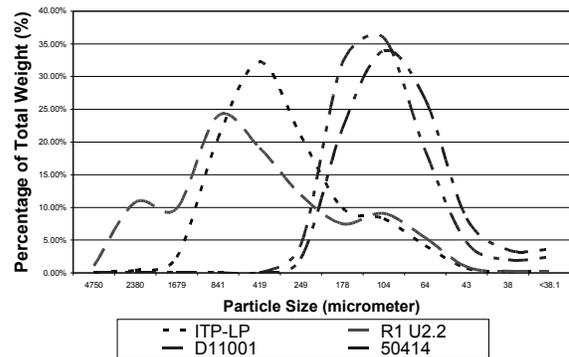
**Figure 6.** Particle-size distribution for low-cost TiCl<sub>4</sub> DuPont and ITP (50414 and ITP LP, respectively) and standard (D11001 and R1 U2.2, respectively) TiCl<sub>4</sub> powders. The distribution indicates a difference for each supplier but no difference for TiCl<sub>4</sub> purity.
