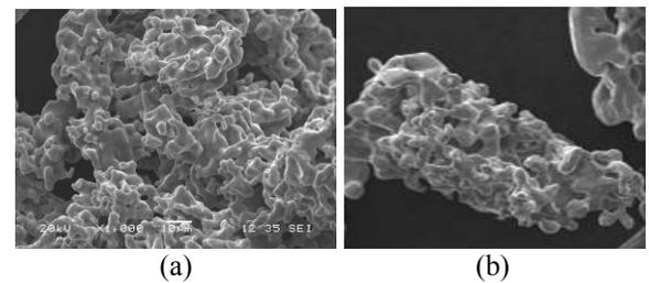
**Figure 5.** DuPont powder produced with high-purity TiCl<sub>4</sub> (a) and low-cost TiCl<sub>4</sub> (b) indicating little change in powder morphology.
