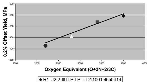
**Figure 9.** Correlation of yield strength and oxygen equivalent for low-cost  $\text{TiCl}_4$  DuPont and ITP, 50414 and ITP LP, respectively, and standard  $\text{TiCl}_4$  powders D11001 and R1 U2.2 for DuPont and ITP, respectively.
