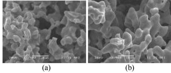
**Figure 4.** ITP powder produced with low-cost ilmenite-based TiCl<sub>4</sub> (a) and standard TiCl<sub>4</sub> (b) indicating little change in powder morphology. Note the ligament type structure in the as-received powders.
