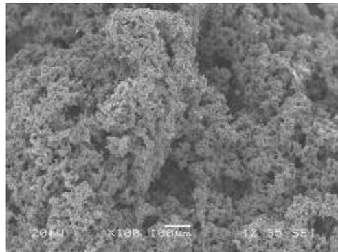
**Figure 10.** Typical as-received ITP powder that exhibits a tapped density of approximately 8% of theoretical.
