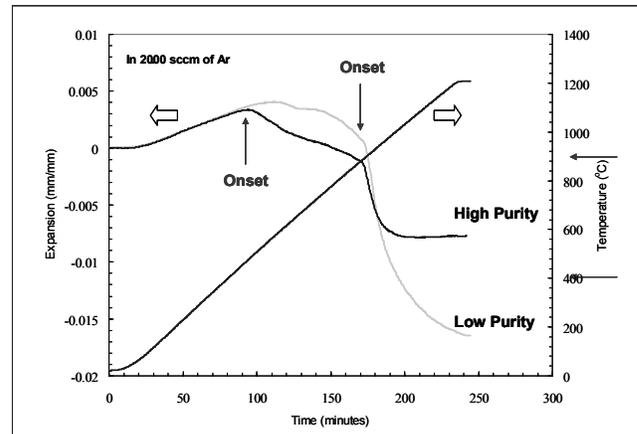
**Figure 2.** Dilatometer curves for the low-purity and high-purity TiCl<sub>4</sub> ITP powders. The presence of trace impurities have altered the onset of sintering and have increased the sinter-start temperature from 400°C to 900°C. The increase from 400°C to 900°C is significant to the decomposition of Na-bearing compounds.
