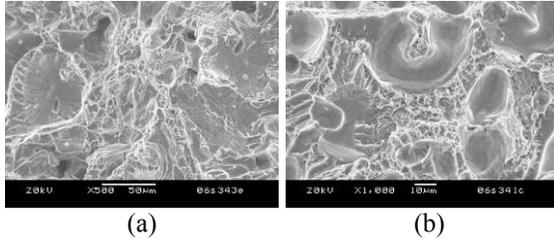
**Figure 8.** Fracture surface of sintered compacts of ITP (a) and DuPont (b) indicating a mixed failure mode of ductile rupture and cleavage. No trace elements were found on the fracture surfaces indicating that the low-cost  $\text{TiCl}_4$  had not adversely affected ductility.
