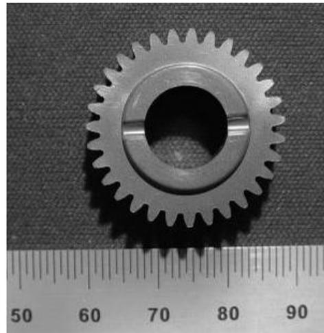
Figure 11. Commercial die-pressing using low-cost TiCl<sub>4</sub> ITP powder.
