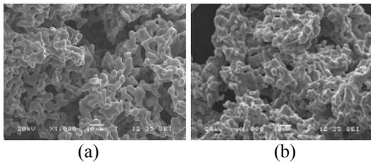
**Figure 3.** Powders produced by ITP (a) and DuPont (b) from low-cost ilmenite-based TiCl<sub>4</sub> showing morphology typical for Na-reduced powders and very similar structure for the two suppliers.
