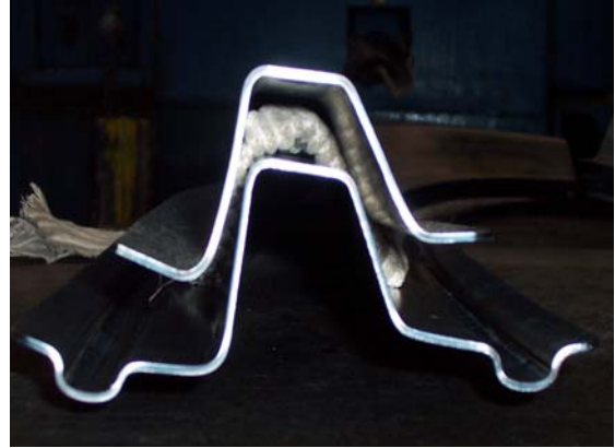
Figure 2. Effect of stretch with four-break lock step. Note that top section was not stretched.
