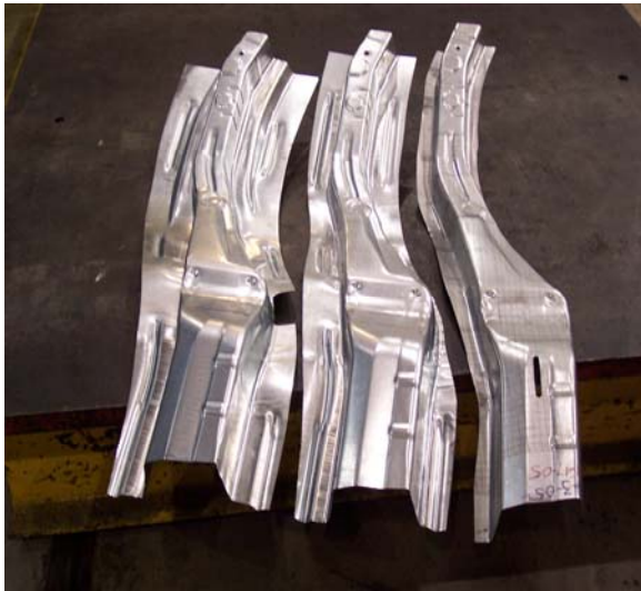
Figure 4. Rail Stampings Three Processes.
