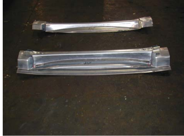
Figure 5. Cowl Cross-Bar Two Processes.
