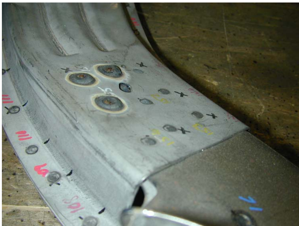
Photo 10. Standard MIG puddle welds were used where RSW guns would not fit into the box section.
