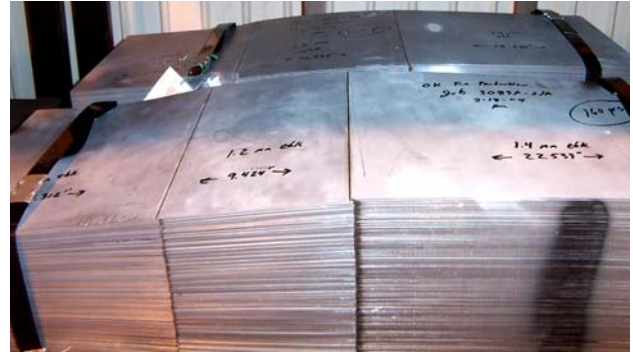
Figure 2. Rail inner and rail outer laser-welded blanks.
