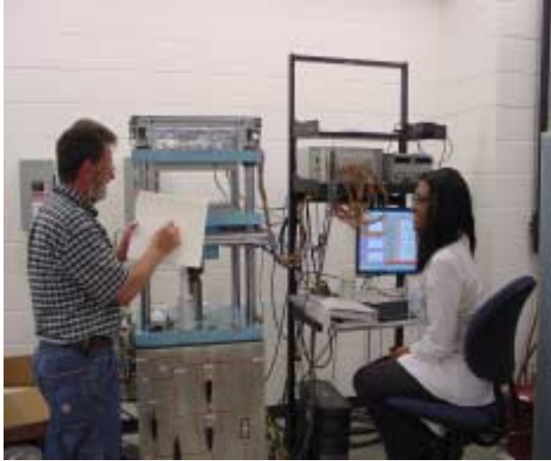
Figure 5. Radial-permeability test rig showing associated data acquisition and monitoring station.
