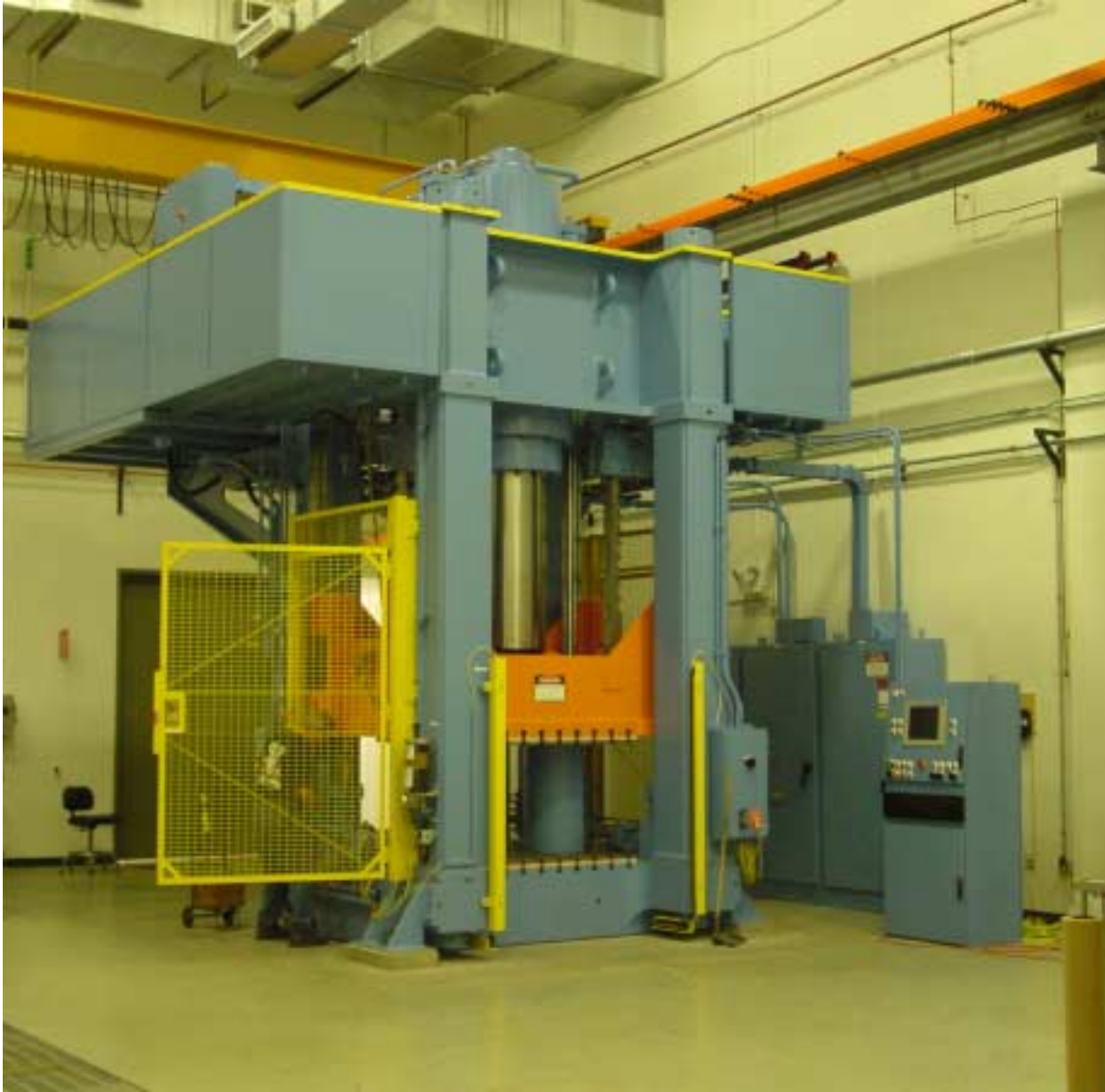
Figure 1. Intelligent-leveling, 750-net-ton, Williams White injection/compression press installed in ORNL composite processing laboratory.
