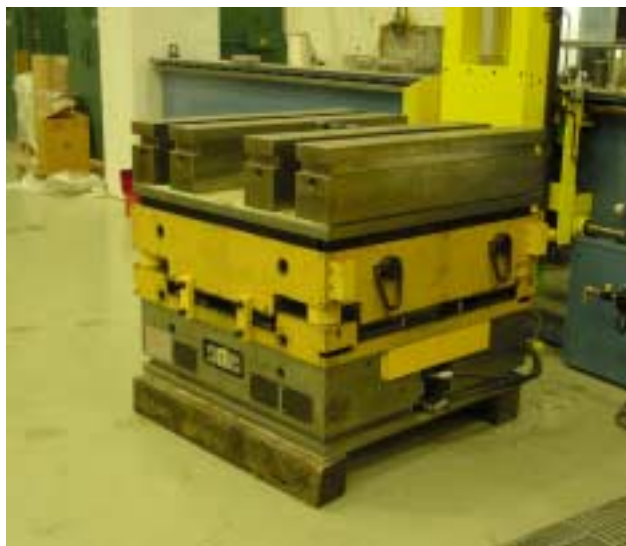
Figure 2. General-purpose flat-plaque mold for SRIM, SMC, and thermoplastics.
