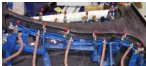
Figure 6. Carbon-fiber assembly in heated bonding fixture.
