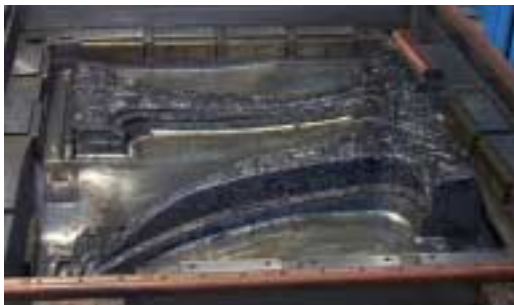
Figure 4. Carbon-fiber B-pillar preforms in the SRIM mold.
