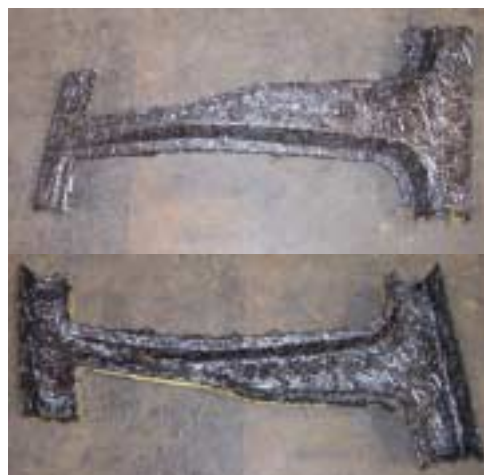
Figure 3. Carbon-fiber B-pillar preform, outer and inner views.
