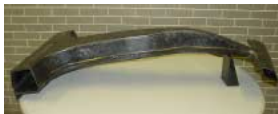
Figure 5. Molded carbon-fiber B-pillar.
