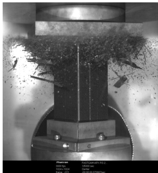
Figure 2. Bonded tube tested at 5000 mm/sec.
