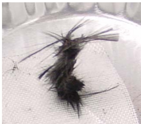
Figure 6. Extracted carbon fiber-and-epoxy plug specimen.
