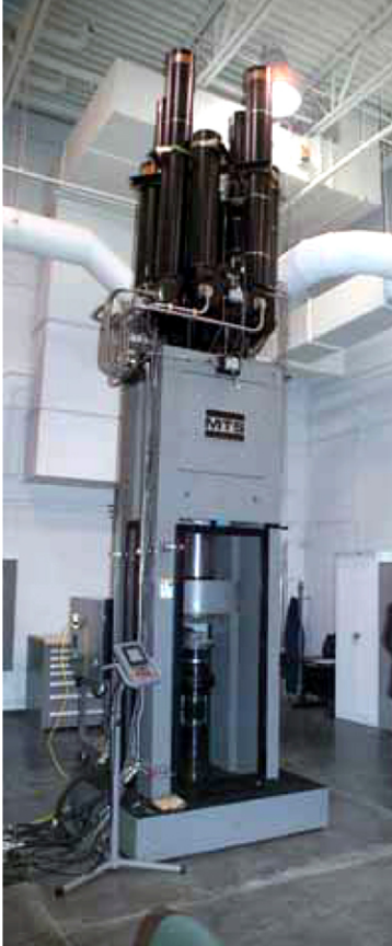
Figure 1. Installation of TMAC in the NTRC.
