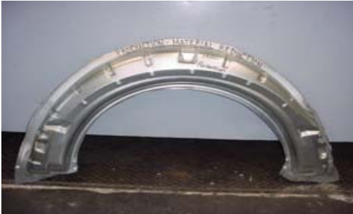
Figure 21. Successful wheelhouse part with reduced production blank.
