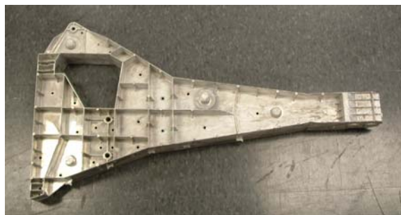
Figure 6. Thixomolded magnesium shotgun casting.
