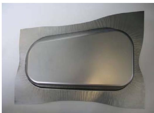
Figure 19. Pan drawn with closed-loop control.
