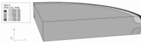
Figure 8. 3D Density distribution for the round cylinder (0.2 inch final height).
