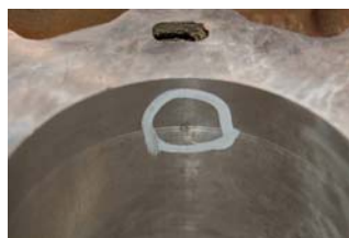
Figure 4. Pinhole porosity exposed by boring.
