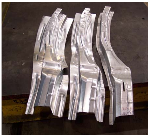
Figure 4. Rail Stampings Three Processes.
