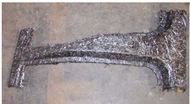
Figure 10. Carbon-fiber preform for B-pillar outer panel.
