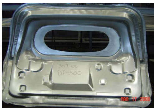
Figure 7. Liftgate panels made from A6111-T4, BH210 and DP500.
