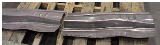
Figure 2. Close-up of a half-sized D steel baseline panel formed on the Common Die.
