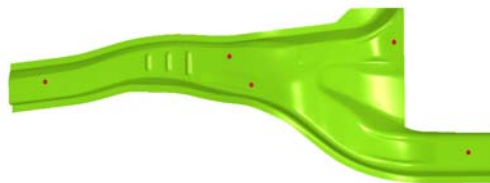
Figure 1. Illustration of Common Die Panel, indicating 5 datum points.
