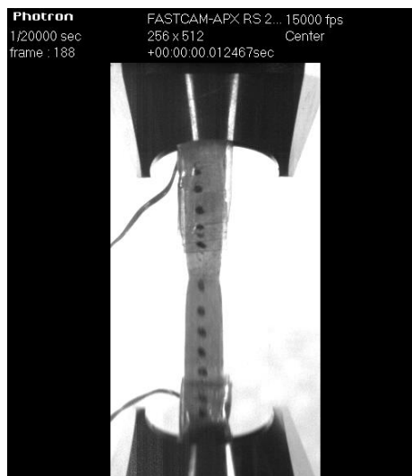
Figure 2. High-rate digital image of a sample right before fracture: deforming at 640 inch/sec under 93°C.
