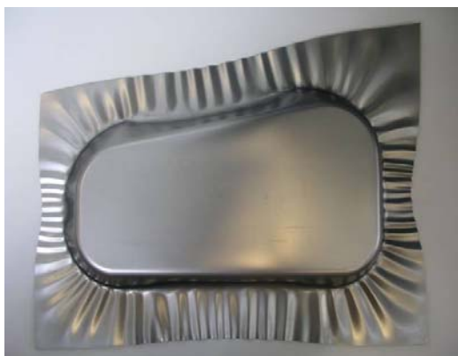
Figure 18. Pan drawn without closed-loop control.
