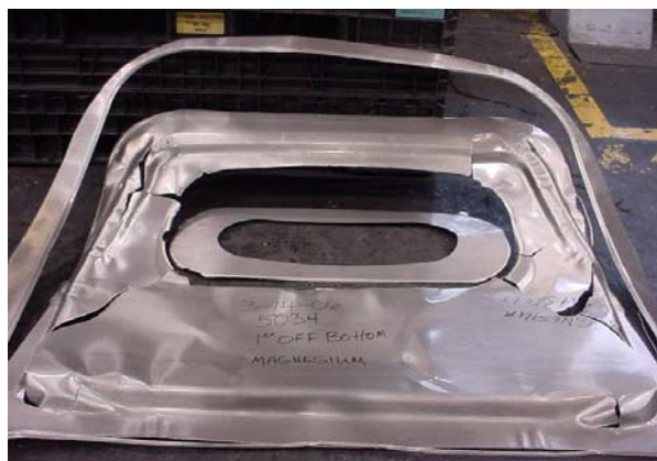
Figure 16. Magnesium AZ31 liftgate trial with 404 lubricant and minimum tonnage.
