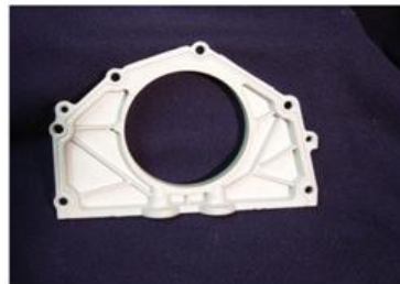
Figure 9. Mg rear oil seal carrier cast by Thixomat.
