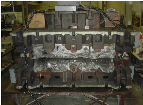
Figure 2. The conventional stamping die refitted for the WF feasibility study performed in Phase I.
