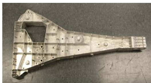
Figure 10. Thixocast AM60 “shotgun.”
