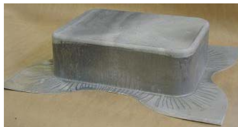
Figure 5. Deep-drawn panels warm formed using a purpose-built warm-forming die.
