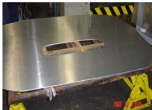
Figure 5. Blank from A6111-T4 used in tryouts.
