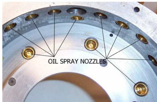
Figure 1. Photo of inside of motor housing showing spray nozzle locations.
