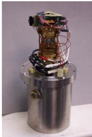
Figure 6. Core of first FY 2006 ORNL prototype inverter.
