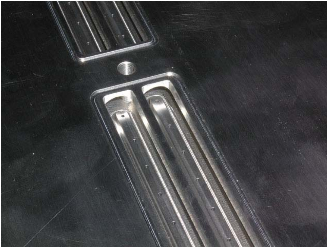
Figure 15. Close view of the nozzles, elongated holes, and O-ring grooves
