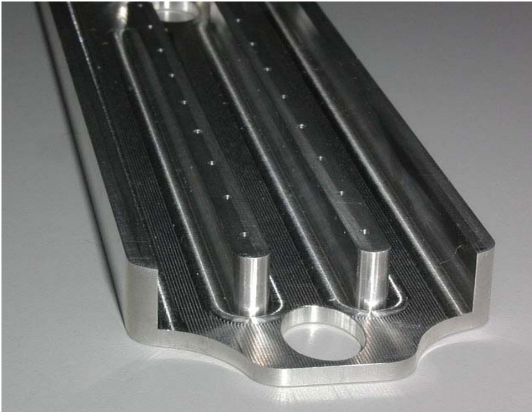
Figure 17. View of one end of the nozzle plate
