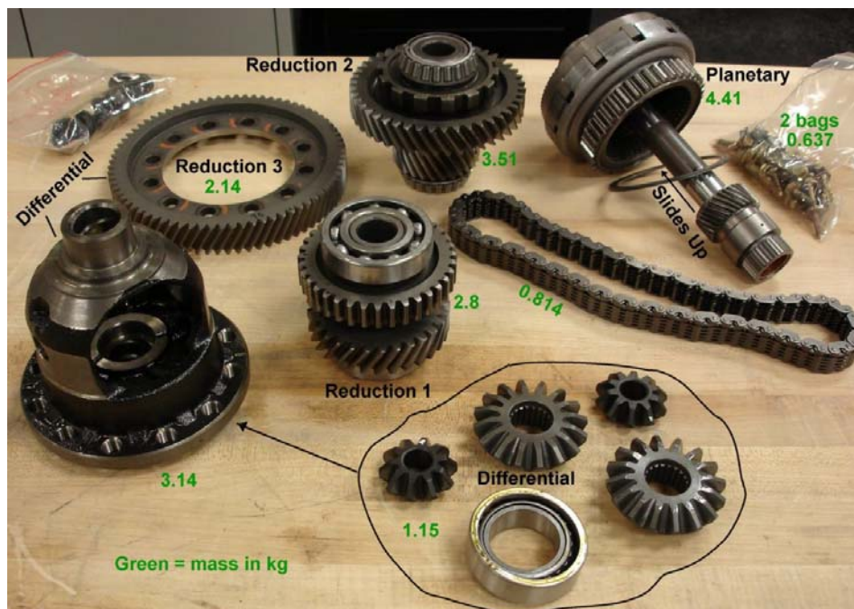
Figure 11. Components making up the Prius gear box.
