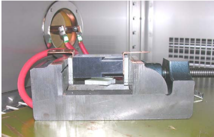
Figure 3. Single Prius film capacitor test set up.
