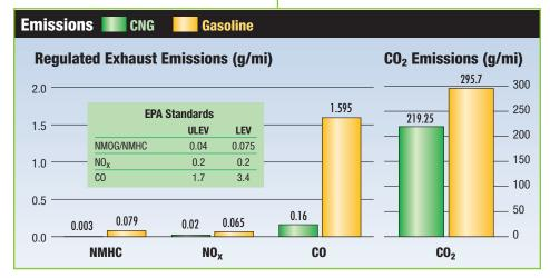
Results from a study conducted by the U.S. Department of Energy, Office of Transportation Technologies, showed greatly reduced emissions in a dedicated natural gas-fueled, 4-cylinder 1998 Honda Civic when compared with those from a comparably equipped, conventional gasoline-fueled Civic.
