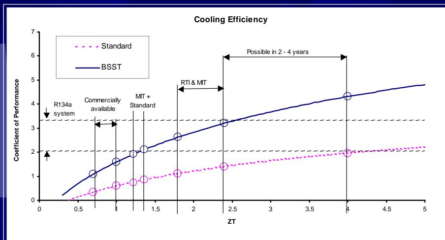
Horizontal band represents the COP for a system using R134a.
