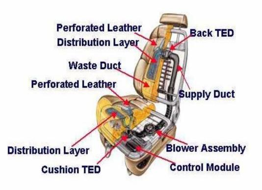
Most successful and highest production volume thermoelectric system in vehicles today
