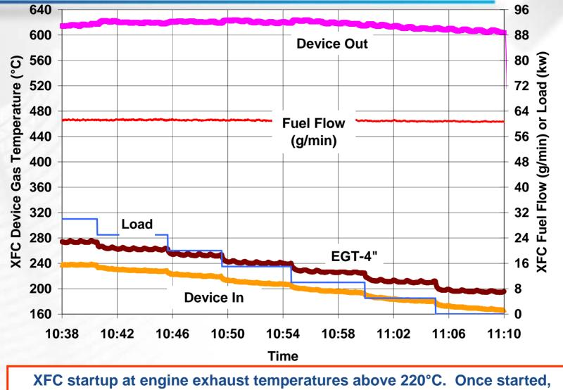
ability to operate at exhaust temperatures as low as 180°C
