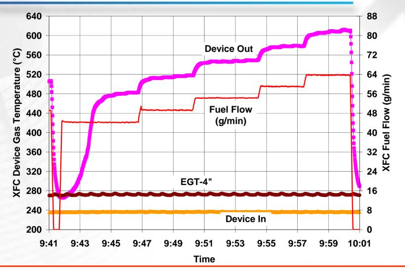
Dodge Ram 40mph: Controlled temperature rise to 610°C inlet to DPF at 236°C inlet to XFC.
