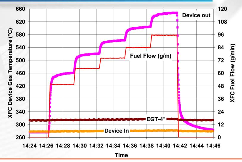
Dodge Ram 70mph: Controlled temperature rise to 650°C inlet to DPF at 270°C inlet to XFC.
