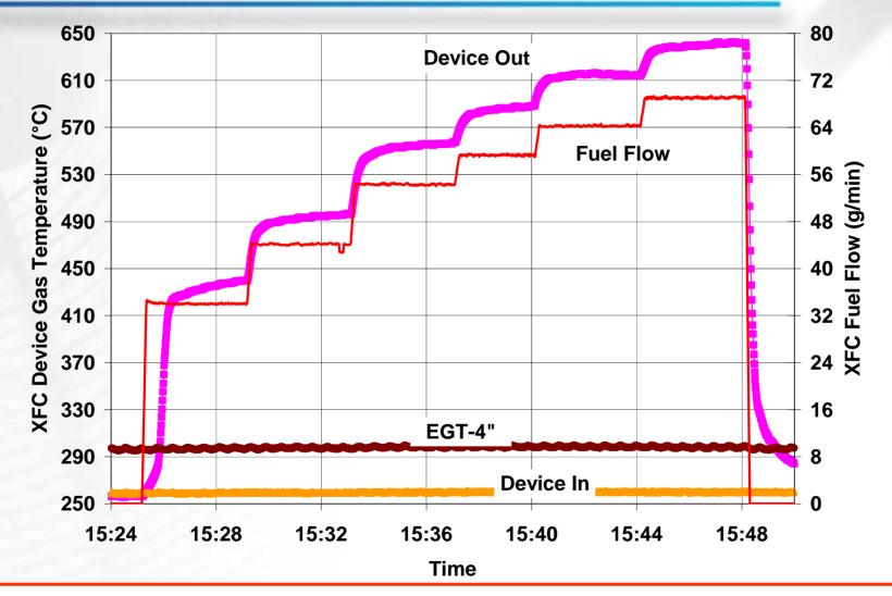
Dodge Ram 55mph: Controlled temperature rise to 650°C inlet to DPF at 255°C inlet to XFC.
