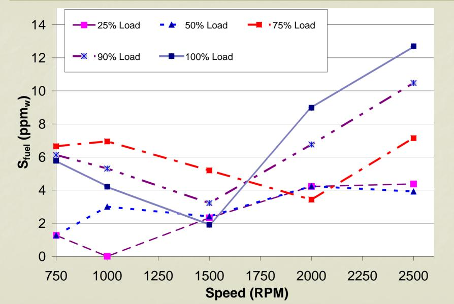
SO<sub>2</sub> exhaust levels measured w/ 1.5% Sulfur Oil and Zero Sulfur Fuel. Typical oil is only .5% S
