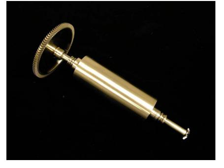
Permanent Magnet rotor Hybrid-Ceramic, selflubricated bearings cooled with F-50.
