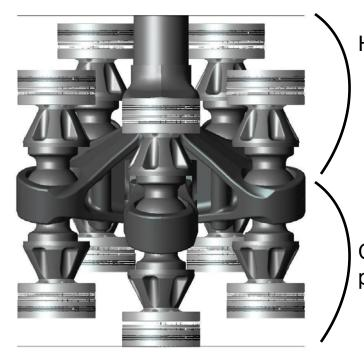
Hybrid pistons Hydraulic Linear alternator Air pump
