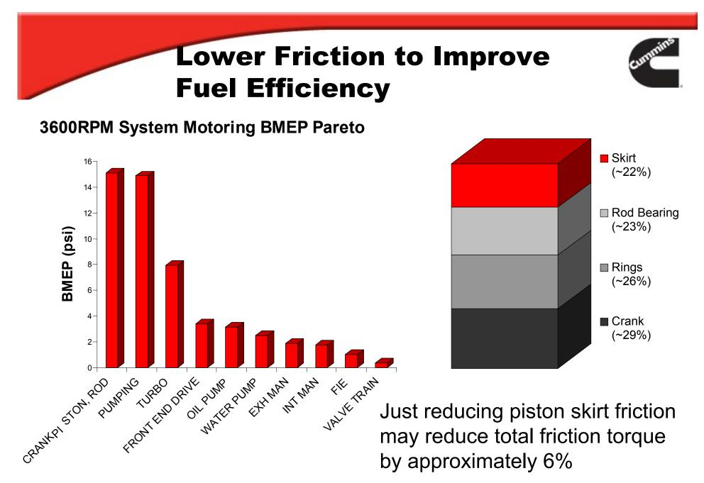
Pareto data normalized I6, V6, & V8 motoring friction test results
