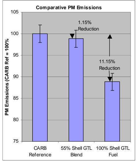
Shell GTL Fuel provides a significant PM emissions reduction over CARB ULSD reference fuel
