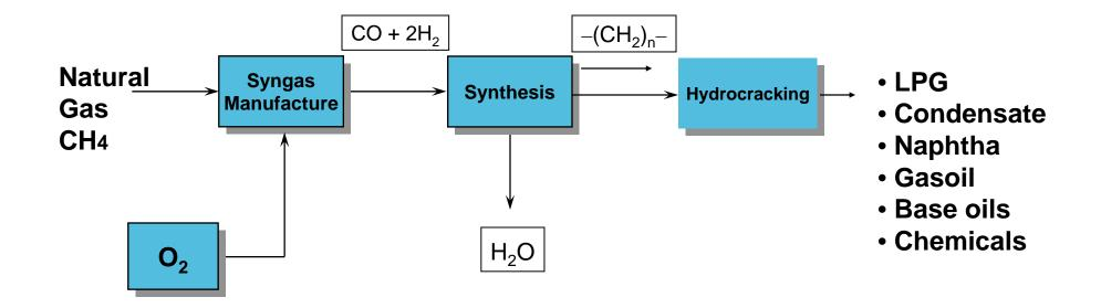
Shell's proprietary process: Shell Middle Distillate Synthesis (SMDS)
