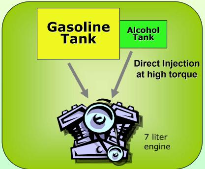
turbocharged, high pressure, high compression ratio
