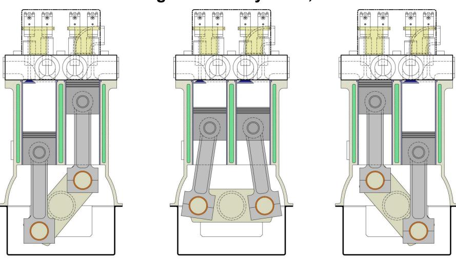
A pivot shaft replaces the crankshaft and oscillates CW then CCW through a range of about 90°.
