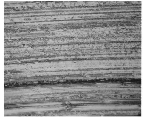
Evidence of abrasive and oxidative wear
