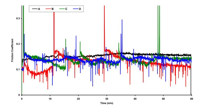
Friction coefficient nearly constant for duration of test for all oils
