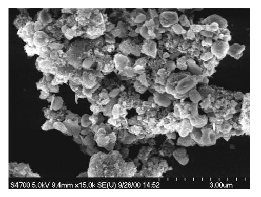
□ Insoluble solid particles in used oil consist of many components.
