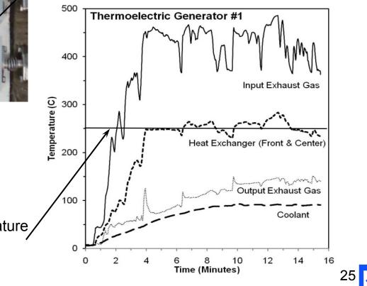
The by-pass valve set point temperature for the heat exchanger was 250°C.
