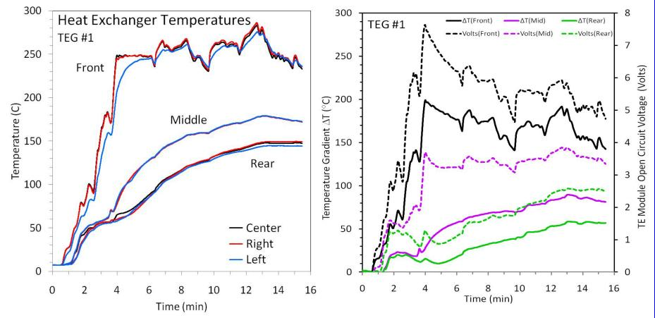
Substantial temperature drop along the length of the TEG: 250°C (Front), 178°C (Middle), and 148°C (Rear)
