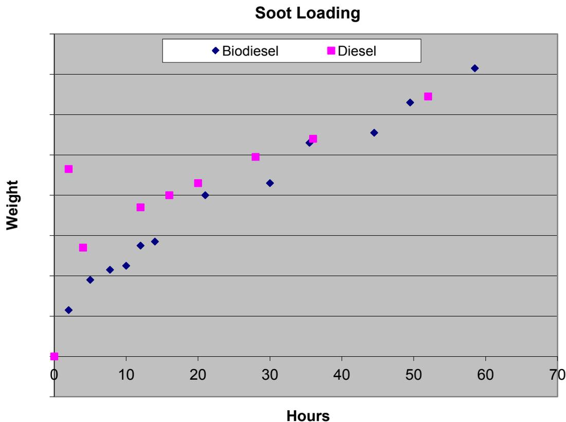
Soot loading cycle was run for 4 weeks to see if the soot loading calibration holds up while on biodiesel.
