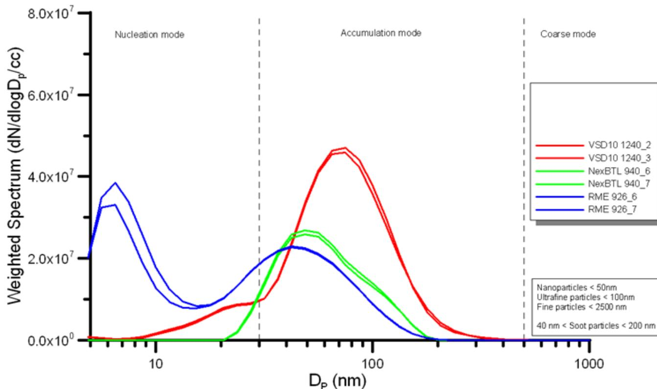
Particle Number (Y-axis) vs Particle Diameter (x-axis)
