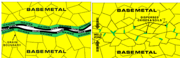
Figure 2. Schematic representation of bond interface before (left) and after (right) ultrasonic welding.
