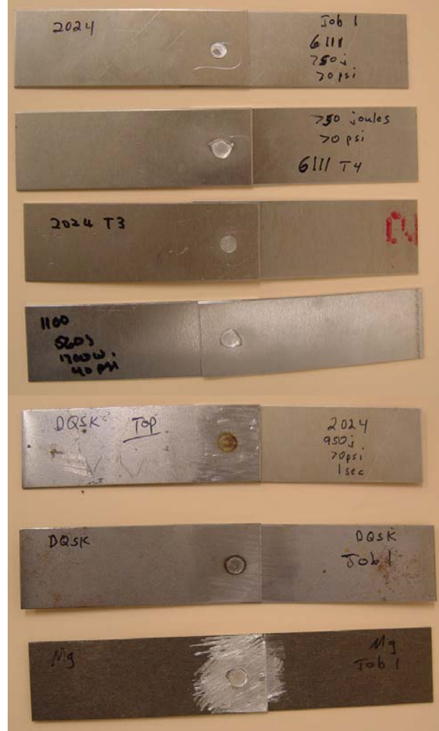
Figure 5. Ultrasonic welds made of various material combinations. From top to bottom: Al2024 to Al6111, Al6111 to Al6111, Al2024 to Al2024, Al1100 to Al1100, DQSK steel to Al2024, DQSK steel to DQSK steel, and Mg AZ31 to Mg AZ31.
