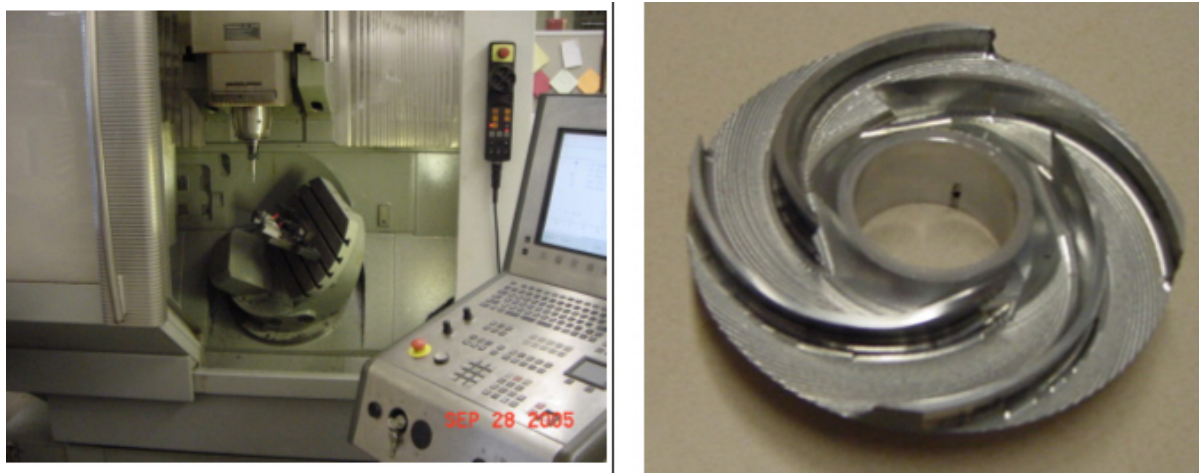
Figure 8. (a) A Deckel Maho DMU50 was the five-axis machining center used for the milling test. (b) One demonstration part was completed by the five-axis machining center.
