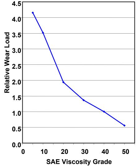
**Normalized Piston - Liner Contact Severity**
