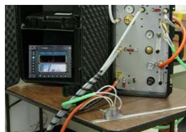
Figure 5. Phased-array probe holder on a test coupon.
