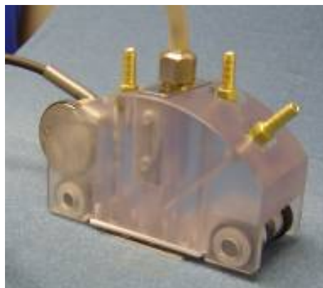
Figure 4. High-frequency phased array embedded in a custom probe holder (Version 1).
