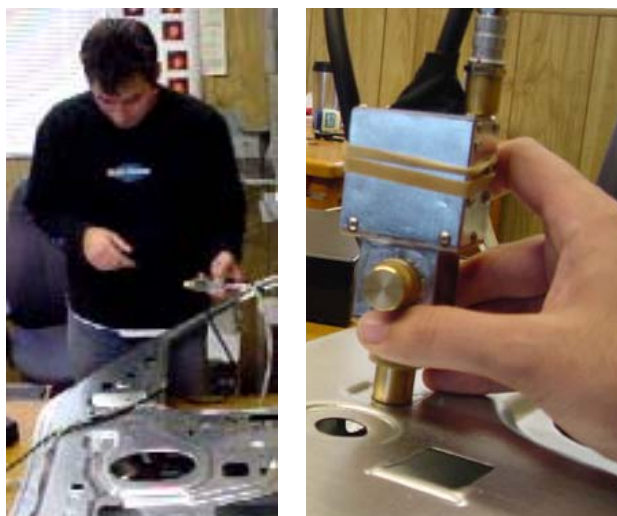
Figure 1. Integrated probe being used to inspect welds on a truck door.
