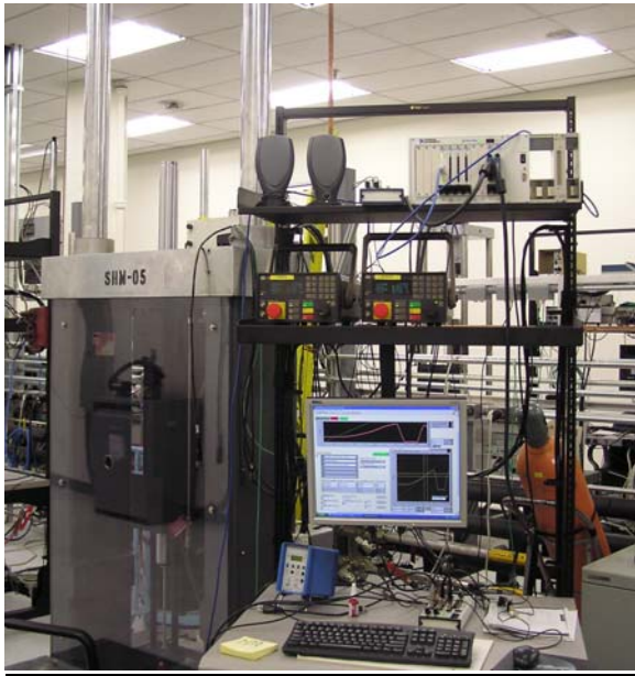
Figure 5. High-rate (18-meter/second) coupon test machine.
