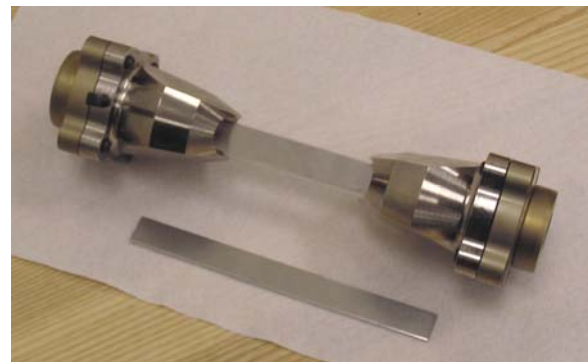
Figure 7. Low-mass grip used in high-rate coupon test machine.
