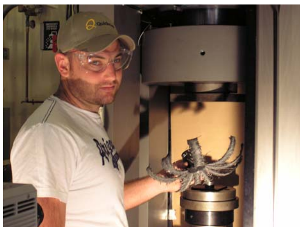
Figure 2. Failed Quickstep tube.
