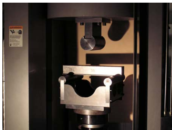
Figure 3. Three-point bend-test set-up on TMAC.
