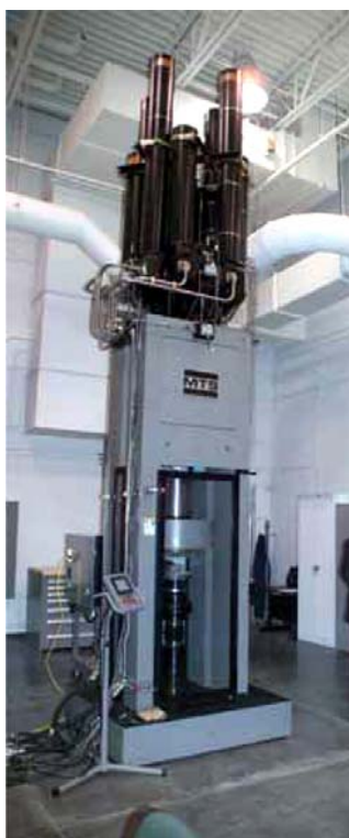
Figure 1. Installation of TMAC in the NTRC composite's lab.
