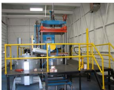
Figure 1. CMI Equipment and Engineering low-pressure casting cell.
