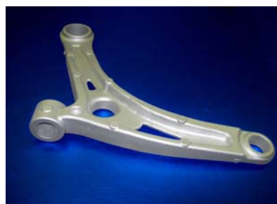
Figure 2. Low-pressure, permanent-mold cast Mg control arm.
