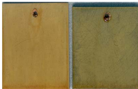
Figure 4. Secondary sealant (organic varnish) provides additional salt-fog corrosion protection. Ferrate conversion coating (left) as compared to reference chromate conversion (right).
