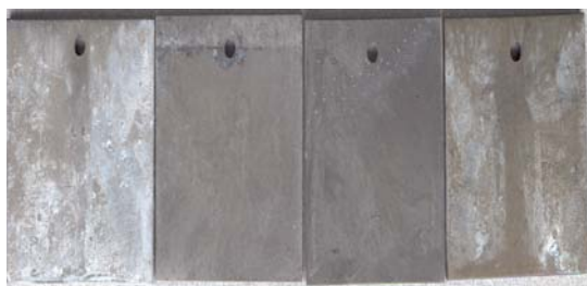
Figure 3. Ferrate with calcium hydroxide bath (two central samples) performed better under corrosive salt-
