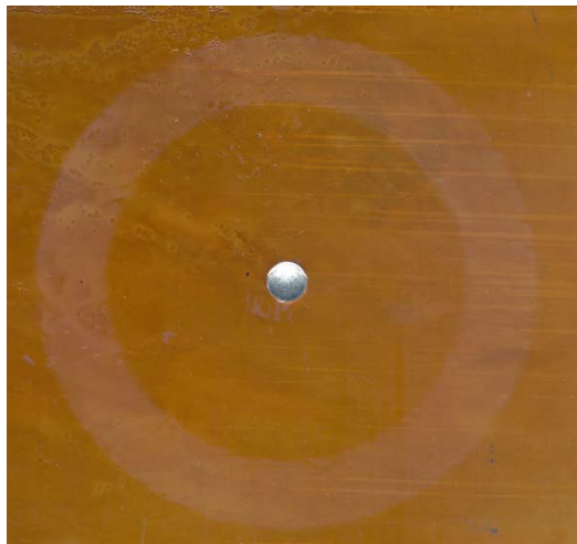
Figure 6. Taber abrasion resistance for organic varnish applied to ferrate-coated Mg alloy.
