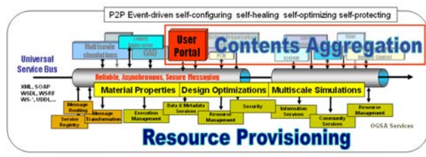
Figure 4. Horizontal software-integration bases on the service-bus concept (as opposed to currently-used centralized, “hub and spoke” architectures leading to vertical silos and stovepipes).
