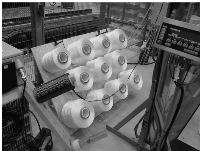
Figure 2. Multi-package creel for in-situ blending experiments.
