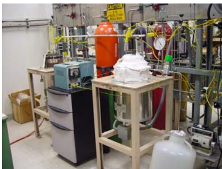
Figure 8. Picture of the PNNL accelerated composite moisture-uptake experimental set-up consisting of two pressure vessels, data logger, etc.
