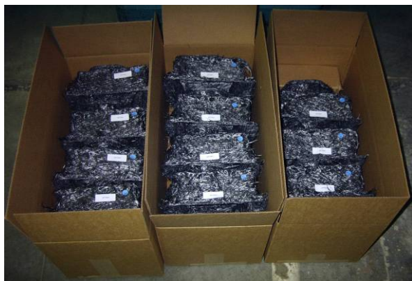
Figure 5. Corvette wheelhouse support preforms were shipped to MFG for molding in polyester.
