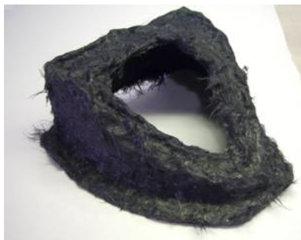
Figure 10a. Corvette preform from reclaimed carbon fiber.
