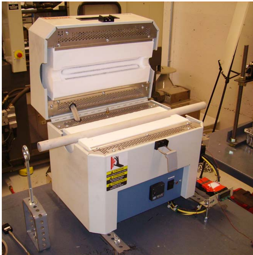
Figure 5. Tube furnace with its top open showing the process tube.
