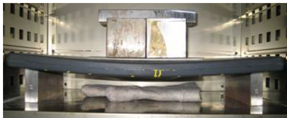
Figure 10. PIM plaque supported along its length (approx. 412.8 mm apart).
