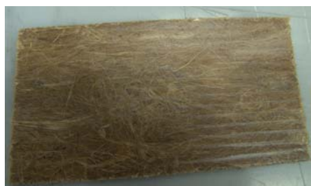
Figure 7. Preform prior to molding with polyester resin, preform in the press (middle) and after molding (bottom).
