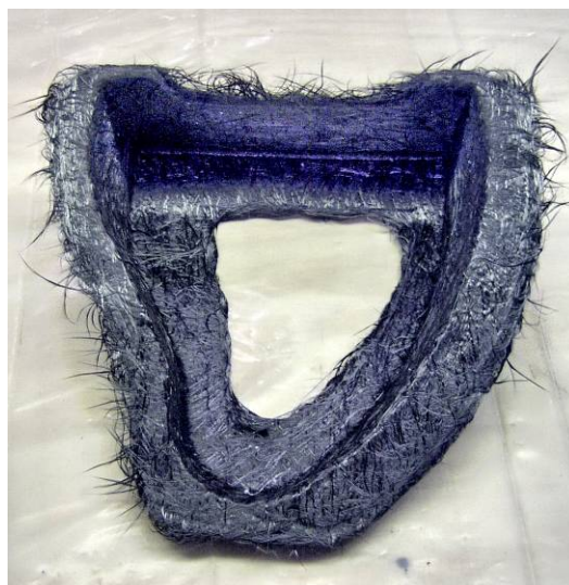
Figure 3. Top and bottom view of Corvette lower wheelhouse support preform in 1-inch chopped carbon fiber. As-formed, no trimming was done.
