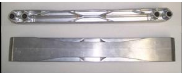
Figure 6. Machined Mg cross members.
