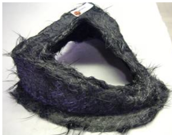
Figure 10b. Corvette preform from virgin carbon fiber.
