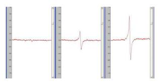
**Figure 3.** ESR traces, with dose increasing from left (unirradiated) to right. Higher peak indicates higher free radical concentration.
