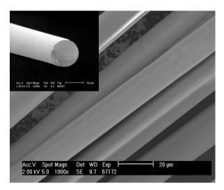
Figure 6. SEM images of lignin precursor fibers.
