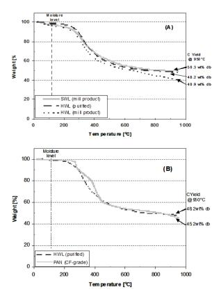
Figure 7. TGA data for lignins (a) and PAN (b).
