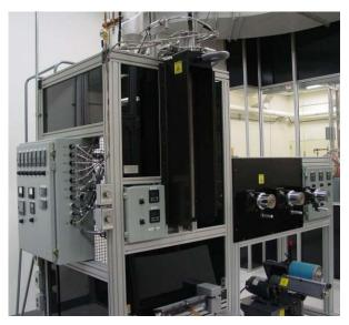
Figure 2. Multifilament melt-spinning equipment.
