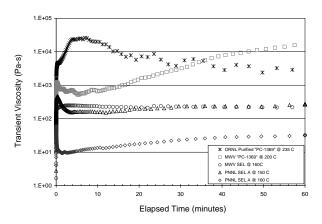
**Figure 3.** Viscosity of HWL as a function of time (at a given temperature).
