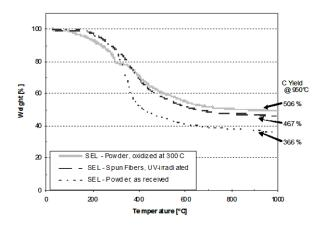
**Figure 8.** TGA data for fibers produced from MWV SEL.
