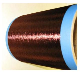
Figure 4. Lignin fiber tow comprising 12 filaments, each 11  $\mu$ m in diameter.
