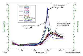
**Figure 3(b).** DSC thermograms of PAN tow, conventionally oxidized in a commercial factory or plasma oxidized in ORNL's multi-zone, single-tow reactor.
