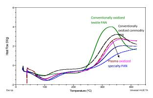
**Figure 5.** DSC thermograms of different PAN fibers oxidized conventionally or by plasma oxidation.
