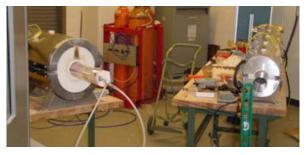
Figure 1. Operation of oxidation and low-temperature carbonization furnaces in precursor evaluation system.
