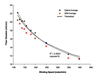
**Figure 5.** Lignin filament diameter as a function of winding speed.
