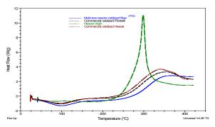
**Figure 4.** Representative DSC thermogram of multi-tow reactor processed oxidized precursor in comparison to those of virgin PAN and commercial oxidized precursors.
