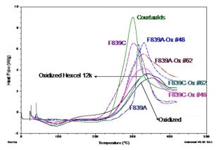
**Figure 2.** DSC characterization of various oxidized textile PAN precursor compositions and comparison to oxidized commercial precursors.
