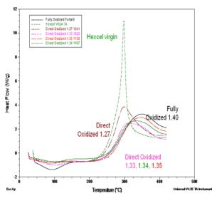
**Figure 2.** Selected DSC thermograms from plasma stabilization experiments.
