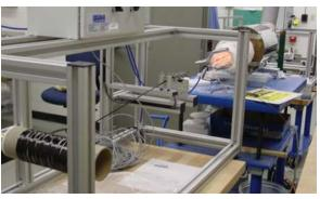
**Figure 6.** Processing of FISIPE precursor using ORNL's precursor evaluation line.
