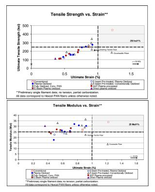
**Figure 1.** Mechanical properties of CFs stabilized and oxidized by various routes then conventionally carbonized at low temperature. There was no tensioning, controlled stretching, or tow spreading during conversion. Conventional data points are for thermally shocked and thermally ramped heating protocols.
