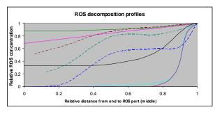
**Figure 2.** Normalized ROS decomposition profiles for various plasma oxidation reactor configurations and thermal conditions.
