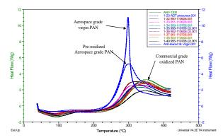
**Figure 3(a).** DSC thermograms of PAN tow, conventionally oxidized in a commercial factory or plasma oxidized in ORNL's multi-zone, single-tow reactor.
