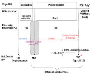
**Figure 1.** Stabilization-oxidation diagram showing the uncertain interface position.
