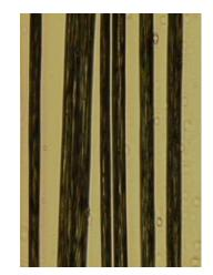
**Figure 7.** Carbon fibers produced from FISIPE precursor.
