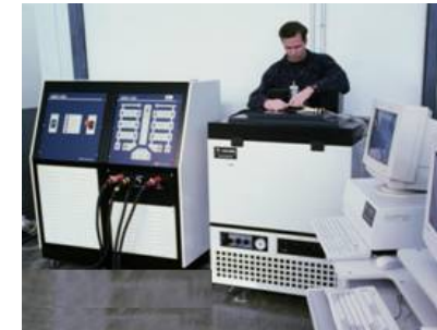
Existing calorimeter between an ABC-150 Cycler & a computer
