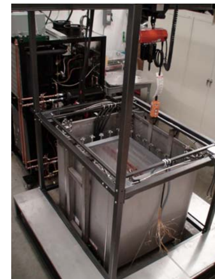
New large calorimeter with heating and cooling system
