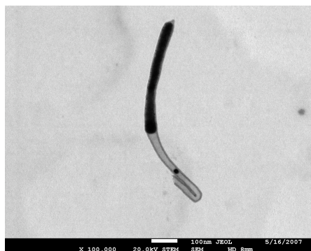
Carbon coating on \text{LiFePO}_4 particle after 100 cycles
