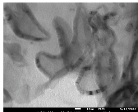
Amorphous carbon fibers in \text{LiFePO}_4 sample
