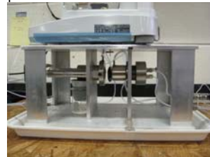
Apparatus for measuring relative permeability of PEMFC GDL's
