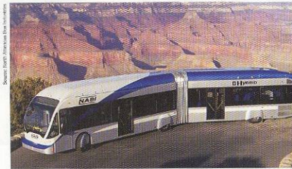
North American Bus Industries (NABI) 60-BRT is a common articulated bus for public transport in major cities. A number of the auxiliary systems, including the air conditioning, are housed on the roof of the bus under access doors similar to that tried in the UAB/NCC project.
