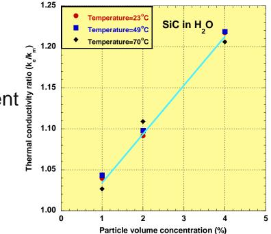
Thermal conductivity enhancement Enhancement level good Increases with concentration No temperature effect beyond H<sub>2</sub>O Nanofluid stability – good Nanofluid agglomeration - minimal
