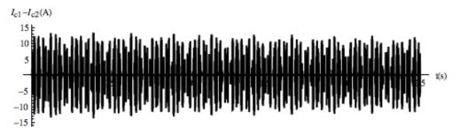
Corresponding electric power difference oscillates with the phase difference at ~14% of the engine frequency. This is the mechanism by which the phases are bound in cyclic motion.
