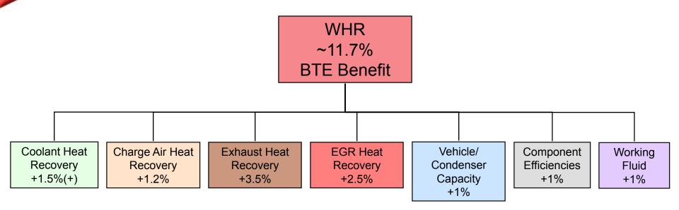
The addition of Coolant and Charge Air heat is done within the existing cooling system capacity
