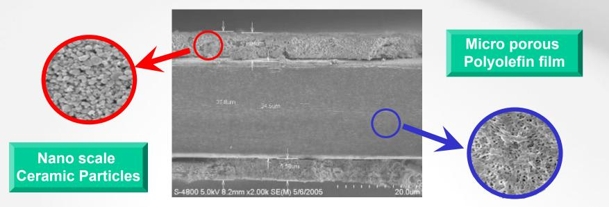
• Has ~6x the puncture strength of conventional separator
