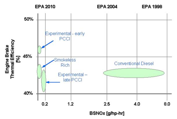
Early PCCI and Smokeless Rich Combustion provide for simultaneous reduction in NOx & PM while maintaining or improving fuel consumption
