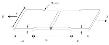
**Butt Weld Test specimen**
