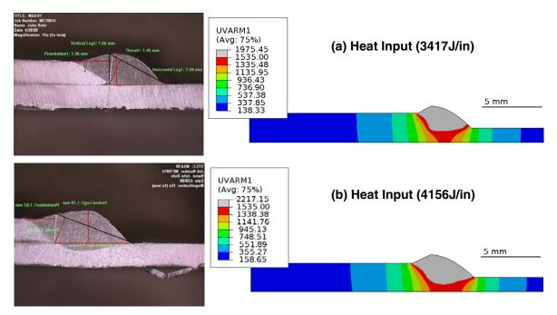
Factors affecting the prediction accuracy included issues with thermal material properties for AHSS and the amount of model calibrations.
