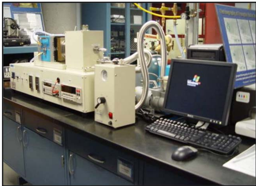
ULVAC ZEM-3 for electrical resistivity and Seebeck coefficient
