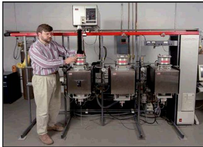
Anter flash diffusivity system for thermal conductivity measurements
