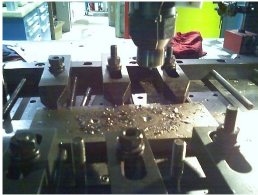
Excessive chip formation observed when no cover plate is used with cast iron.
