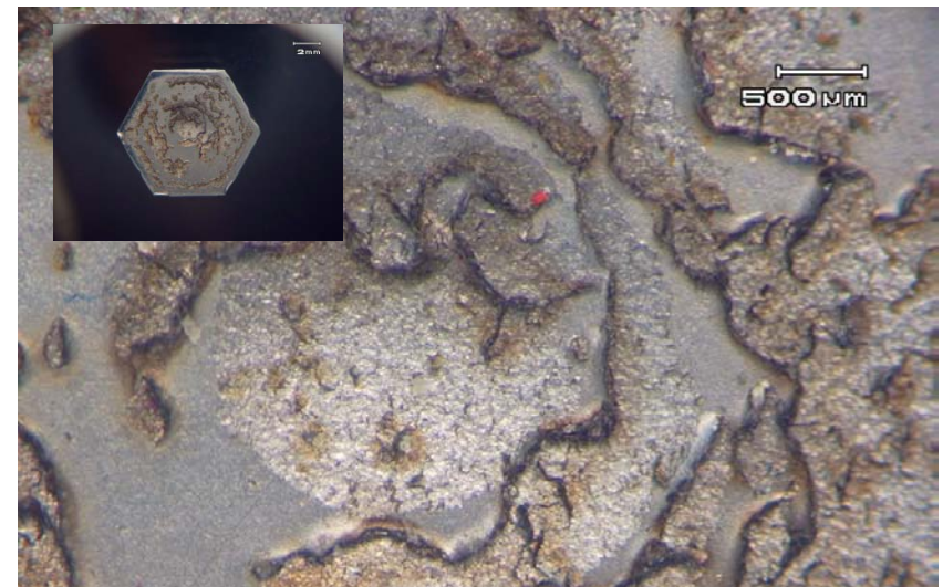
Image of polished steel sample illustrating cavitation erosion induced by ultrasonic agitation
