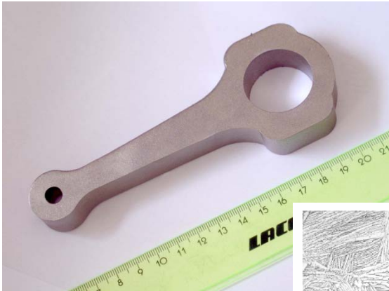
Fine as-sintered grain size
