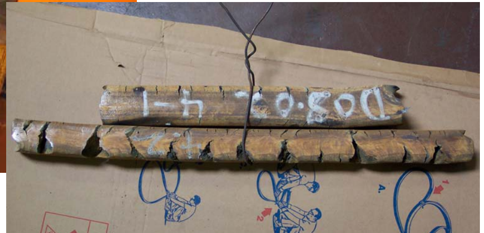
Excessive cracking in Ti6Al4V that was ultimately corrected
