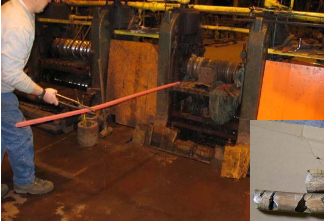
Successful rod rolling of solid state processed Ti1Al8V5Fe beta alloy
